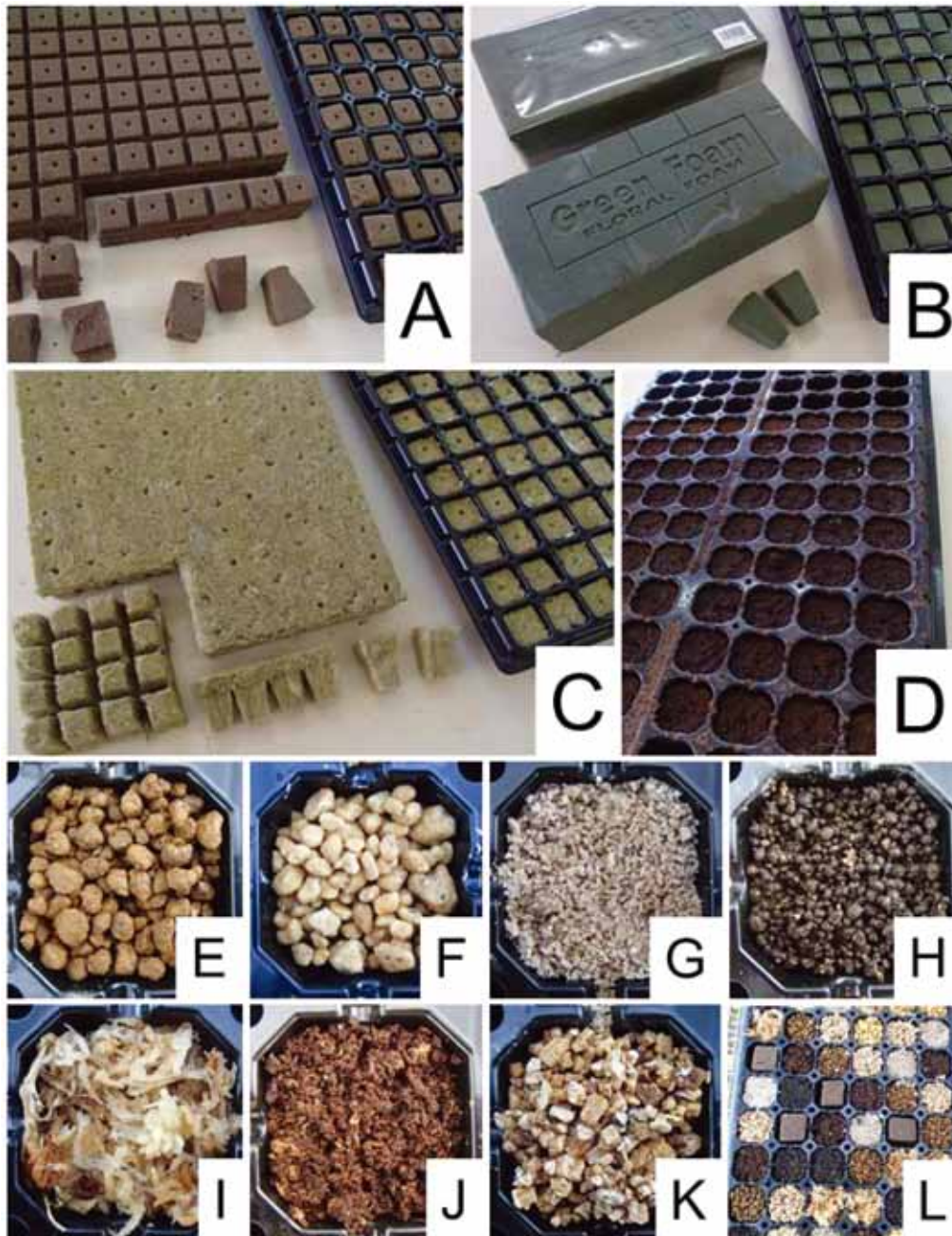
Fig. 3. Examples of rooting media tested in the present study. A-D, artificially-formed media put in 128-cell plug trays [A, phenolic resin foam for plant propagation (Oasis® Rootcubes® P1) ; B, phenolic resin foam for flower arrangement (Green Foam) ; C, rockwool (Grodan® 1" A-OK Starter Plugs) ; D, formed soil (Plant Plug® 128) ]. E-K, non-formed media put in single cells of 72-cell plug trays [E, Akadama soil; F, Kanuma pumice; G, river sand; H, rice nursery soil (Kumiai Baido) ; I, sphagnum moss; J, peat moss; K, vermiculite]. L, an example of 72-cell plug tray in which several media were put in a randomized order. See Table 1 for further information on the rooting media.
